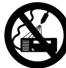
Never direct the high-pressure jet or water hose against the machine itself or against other electrical appliances – **danger of short-circuiting!**
