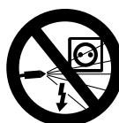
Never direct the high-pressure jet or water hose against electrical equipment, connections and power cords – **danger of short-circuiting!**
